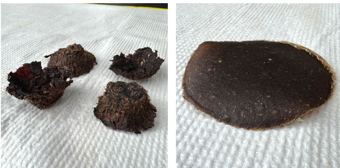
Figure 2 – Examples of biomaterials made from banana peels in this lesson. Left – carton procedure using potassium metabisulfite pre-treatment and drying/curing in a silicone cupcake mold. Right – film procedure with acetic acid pretreatment and drying/curing in a silicone petri-type dish.
